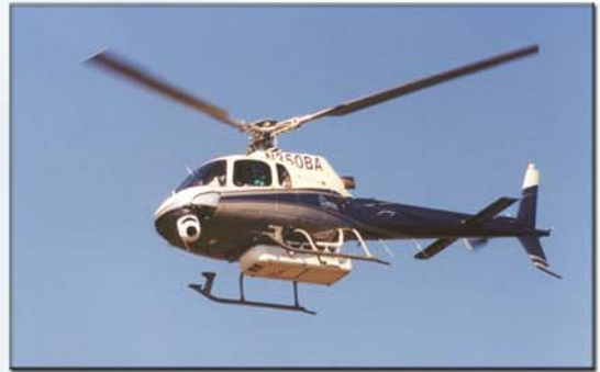
One of Aerotec's two AS350 helicopters, equipped with the Saab TopEye lidar survey system, video cameras, and black-and-white camera
